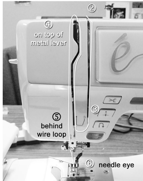
Figure 12. Threading the machine
